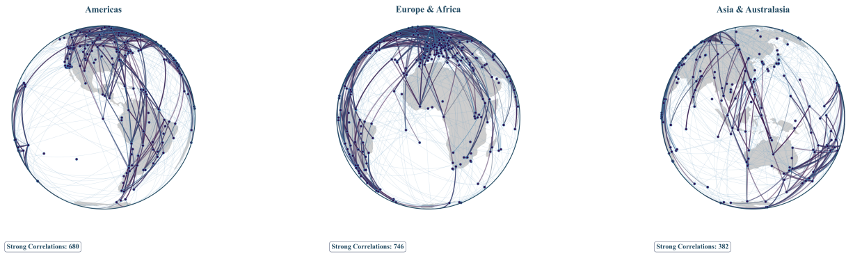
Figure 5. Global Station Correlation Network: Visualization of high-coherence connections across the global GNSS network, revealing directional patterns and spatial anisotropy in timing correlations across intercontinental distances.
